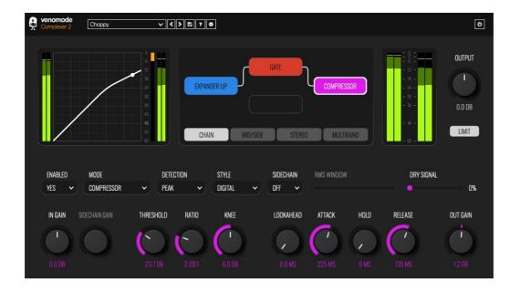
Complexer 2 is a multi-stage dynamics processor, featuring three independently controlled dynamics processors, each with a choice of six different modes.
